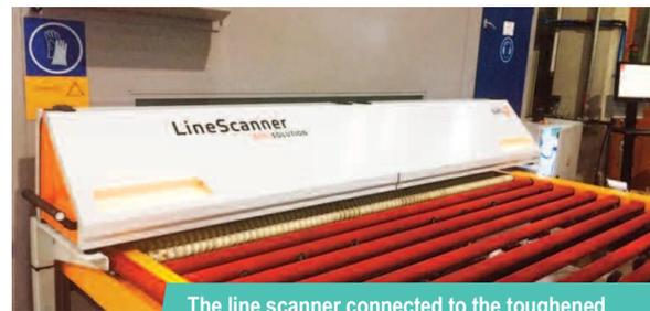
The line scanner connected to the toughened glass furnace [www.glass-iq.com](http://www.glass-iq.com)
