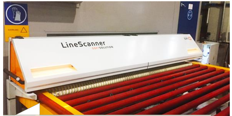
Figure 02: The scanner, directly positioned at the outlet of the tempered furnace, can not only detect stress curves in the glass but also defects as well as the pane format.
